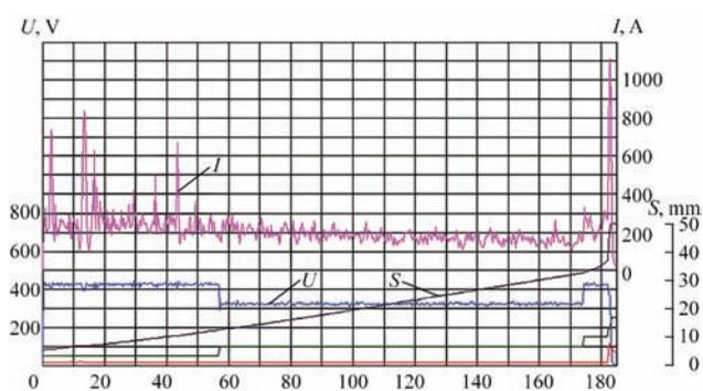
Figure 2. Typical program for changing basic parameters during welding rails using continuous flashing
