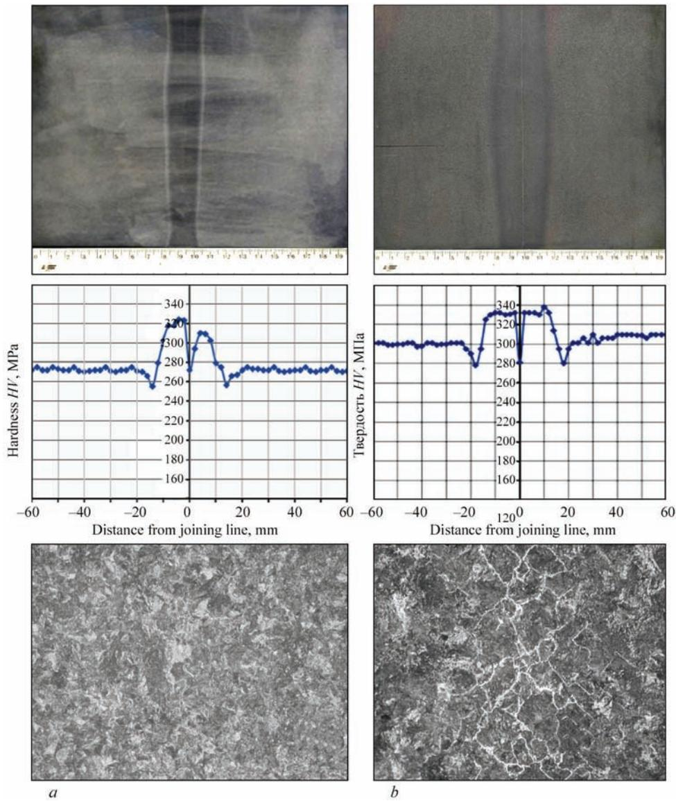
**Figure 10.** Macro-, microstructure ( $\times 100$ ) of hardness distribution ( $HV$ ) of welded joints of R260 rails with different heat input:  $a$  —  $T_w = 65-75$  s;  $b$  —  $90-100$  s
