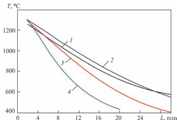
**Figure 6.** Temperature distribution in the HAZ before upsetting during welding of R65 rails at different modes: 1 — with pre-heating ( $t_w = 200\text{--}250$  s); 2 — CF with programmed voltage drop ( $t_w = 180\text{--}220$  s); 3 — PF ( $t_w = 110\text{--}120$  s); 4 — PF ( $t_w = 60\text{--}70$  s)
