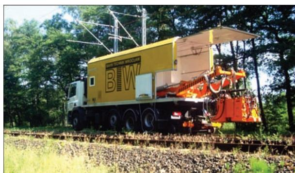
Figure 19. Mobile rail welding complex KSM 007 with welding head K922-1 based on a Volvo machine
