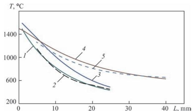
**Figure 7.** Temperature distribution in the HAZ before upsetting during welding R65 rails with different values of current and flashing duration: 1 — PF at  $T = 60$  s,  $I = 370$  A (calculated); 2 — PF at  $T = 60$  s,  $I = 370$  A (experimental); 3 — PF at  $T = 60$  s,  $I = 450$  A (calculated); 4 — CF at  $T = 180$  s,  $I = 170$  A (calculated); 5 — CF at  $T = 180$  s,  $I = 170$  A (experimental)
