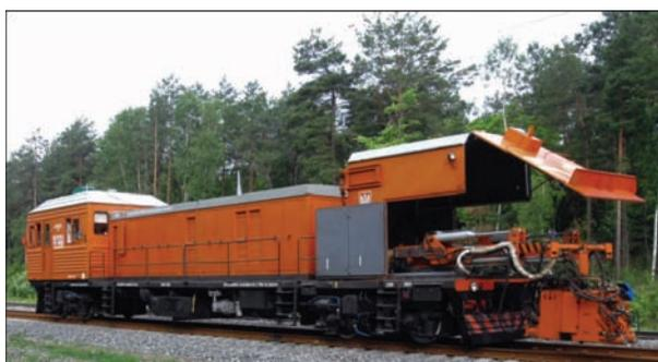
Figure 20. Mobile rail welding complex KRS-1 with welding head K922-1
