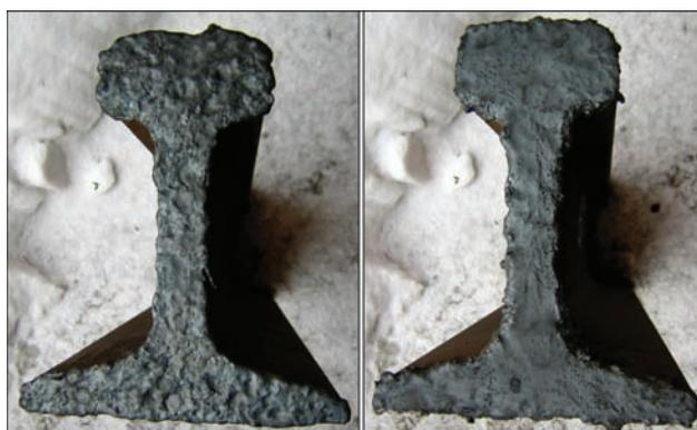
**Figure 8.** Surface of flashing rail ends before upsetting
