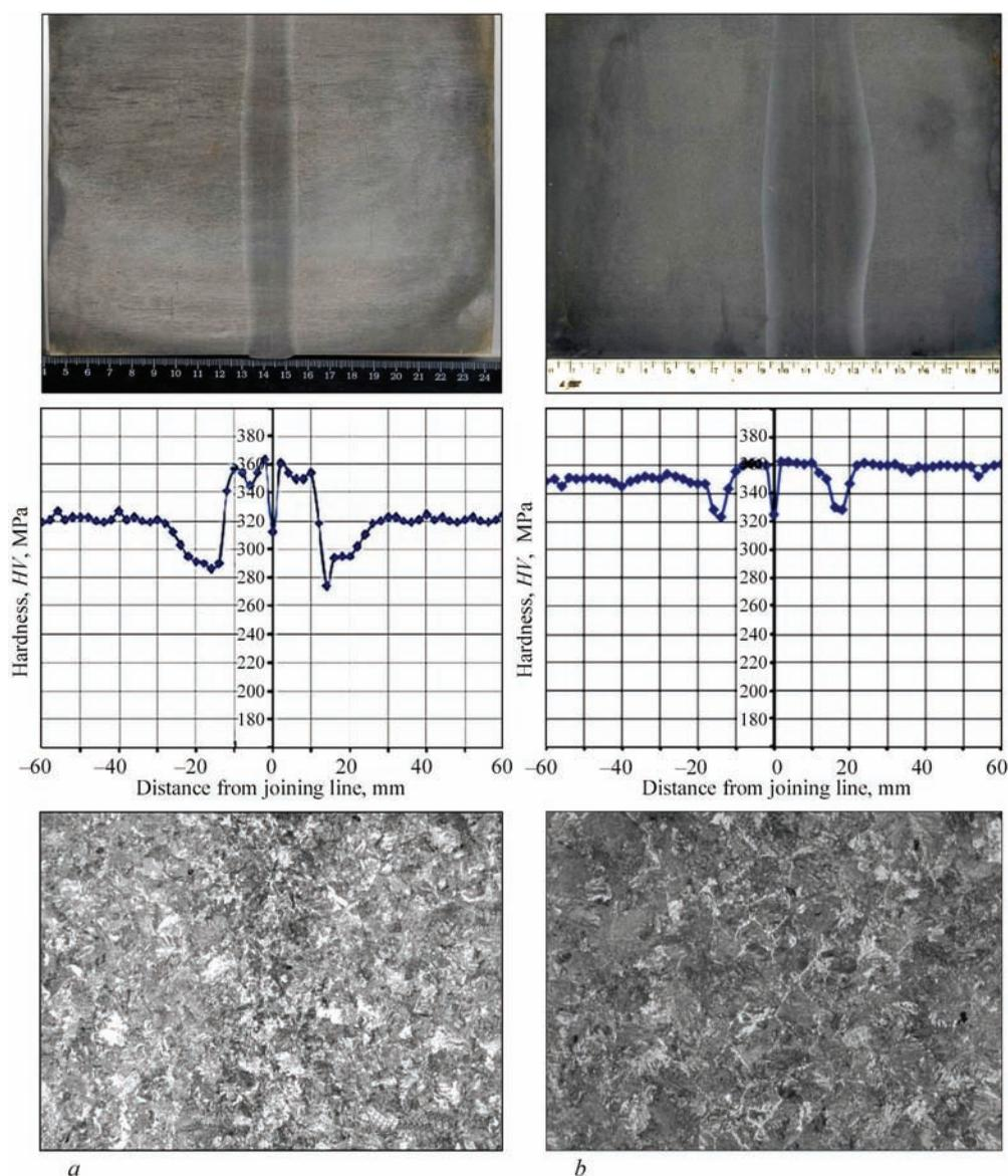
**Figure 12.** Macro-, microstructure ( $\times 100$ ) and hardness distribution ( $HV$ ) in the welded joint of rails of grade R350NT with different heat input: *a* —  $T_w = 65\text{--}75$  s; *b* —  $90\text{--}100$  s
