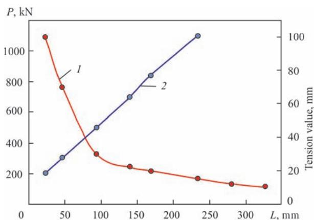
**Figure 15.** Dependence of tension forces ( $I$ ) and tension value (2) of travel of moving clamp of the machine on the length of the jointing section of the rail fastening on the cross-ties at  $\Delta T = 30$  °C
