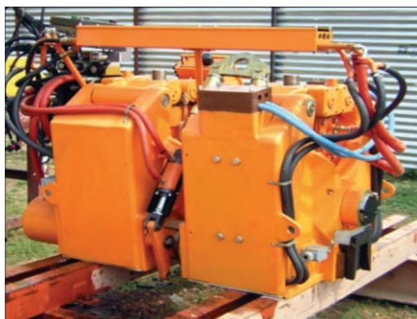
Figure 3. Mobile rail welding machine K900
