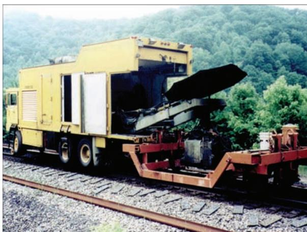
Figure 21. Mobile rail welding complex (USA)
