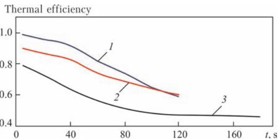
**Figure 4.** Dependence of thermal efficiency on flashing duration at PF (1, 2) and CF (3): 1 — 120 s,  $I$  — 450 A; 2 — 120 s,  $I$  — 370 A; 3 — 180 s,  $I$  — 170 A
