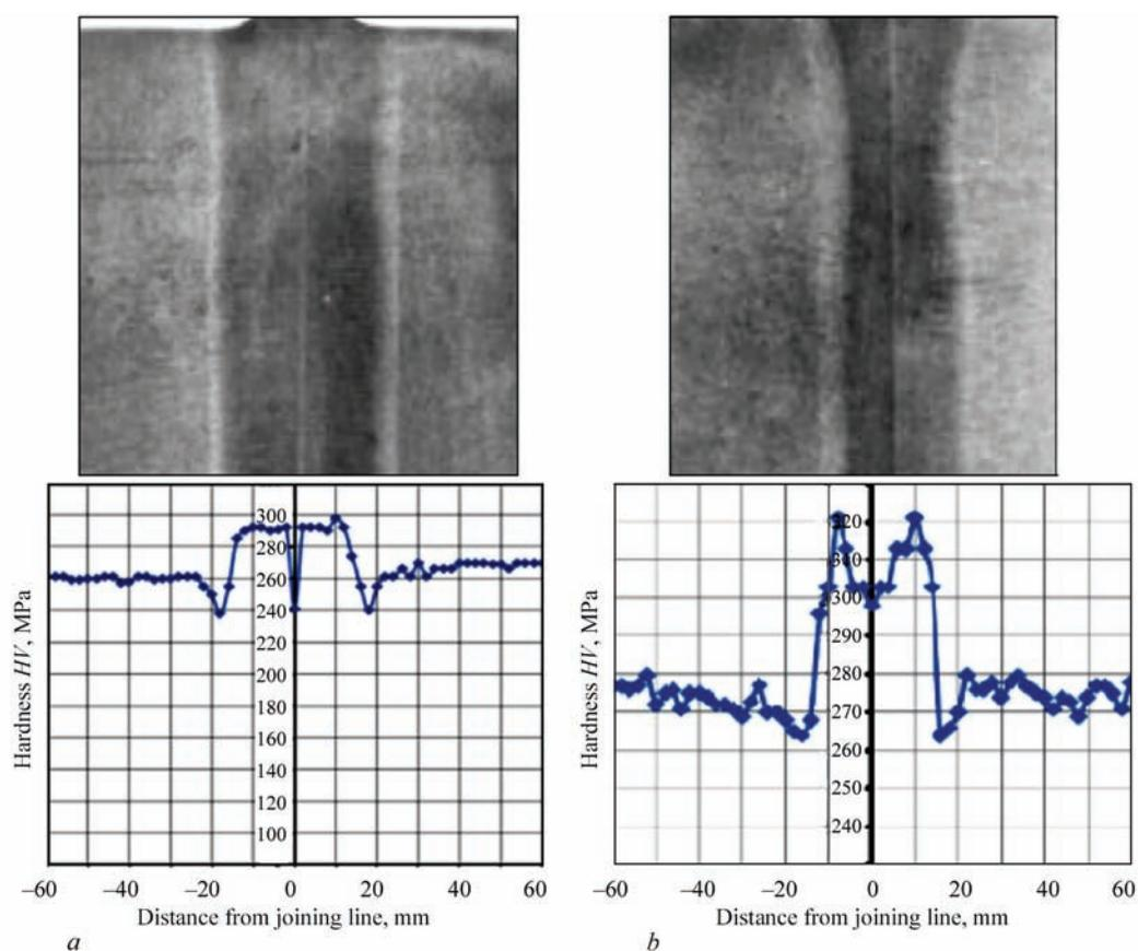
**Figure 9.** Macrosections during flashing of welded joints of rails M76, using CF (a) and PF (b)
