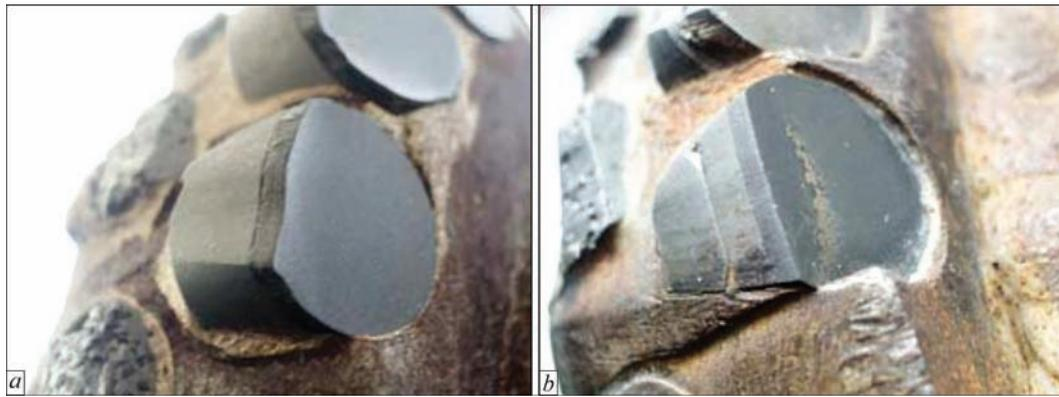
**Figure 1.** Appearance of worn cutters of steel drilling bit blade ( $\times 3$ ): *a* — «Syndrill» DHC after 1000 m drifting; *b* — complex cutter of DHP of ISM of NASU after 250 m drifting
