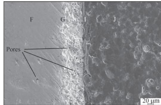
**Figure 5.** Microstructure of complex DHP (ISM of NASU): F — hard-alloy substrate, (G, H, I) — transition zone, J — diamond layer
