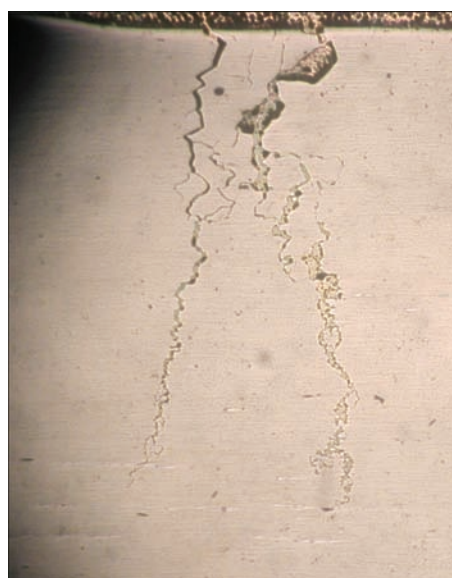
Figure 1. Microstructure ( \times 50 ) of metal of fusion zone of high-tin bronze and steel with ICP of bronze into steel
