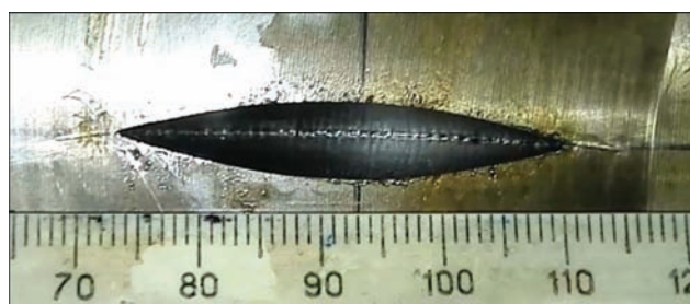
Figure 4. «Whiskers» at the crack tips from the notch side before reaching the opposite surface
