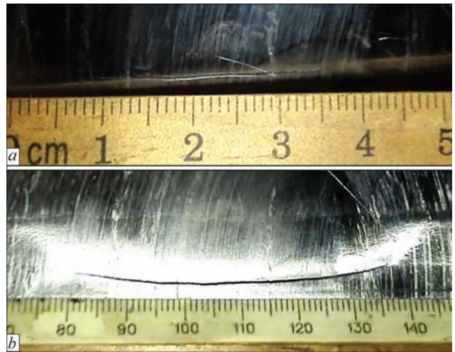
Figure 3. Fatigue crack propagation: growth under plane strain conditions (a) and formation of steel contraction across the sample thickness at the tips of through-thickness crack at its length 2a \geq 35 mm (b)
