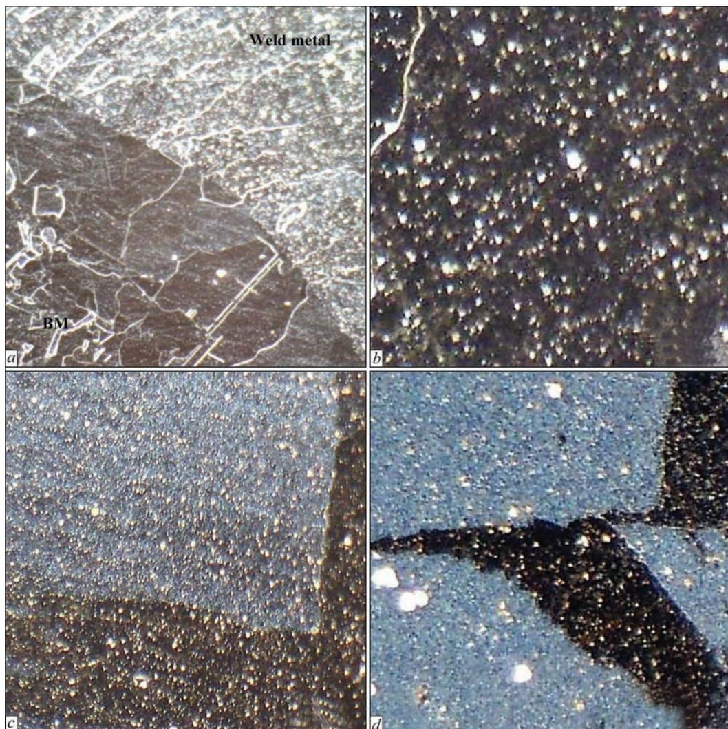
**Figure 4.** Microstructure (*a* —  $\times 200$ ; *b-d* —  $\times 500$ ) of welds (photo in dark field): *a* — transition area «heat affected zone–weld metal», LW,  $v_w = 90$  m/h; *b* — weld metal, EBW,  $v_w = 90$  m/h; *c* — weld metal, LW,  $v_w = 90$  m/h; *d* — weld metal, LW,  $v_w = 180$  m/h
