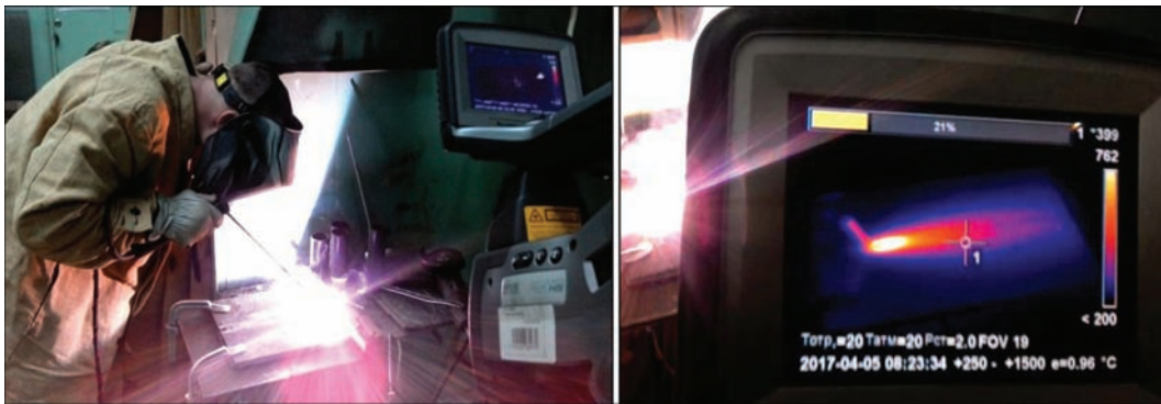
Figure 9. Thermal imaging of temperature fields on the plate surface in downhand welding
