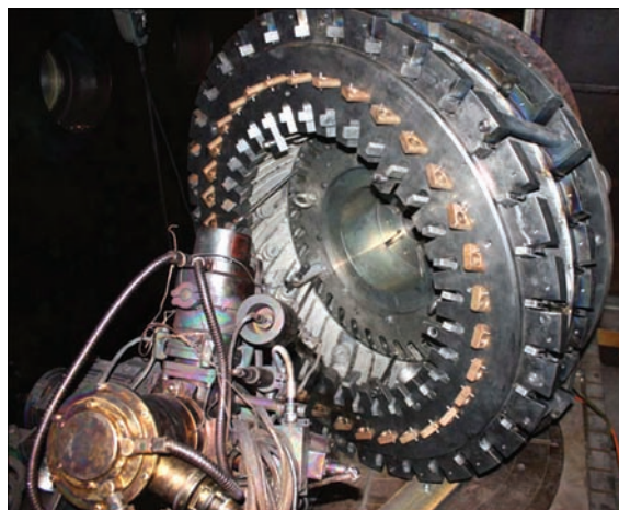
Figure 15. Body of MPC in the rigging for longitudinal welding (in the plane Z-X) of inner welds by inclined electron beam
