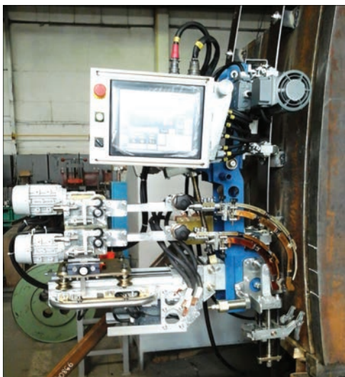
Figure 2. Two-electrode ASH 115M2 machine for ESW of position circular and curvilinear butts joint of 40–200 mm thickness
