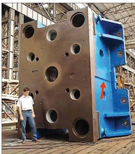
Figure 5. Welded billet of the hydraulic press beam. Billet weight is 150 t, cross-section of a weld (shown by an arrow) made by ESW with consumable nozzle, is 2490×3860 mm
