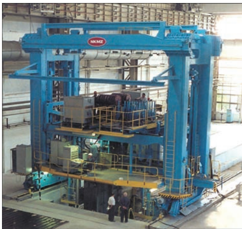
Figure 4. Appearance of an installation for ESW with consumable nozzle for joining metal, the cross-section of which can reach the dimensions of 4000×6000 mm. (G.Z. Voloshkevich Section of ESW of thick metal at PJSC «NKMZ», Kramatorsk)
