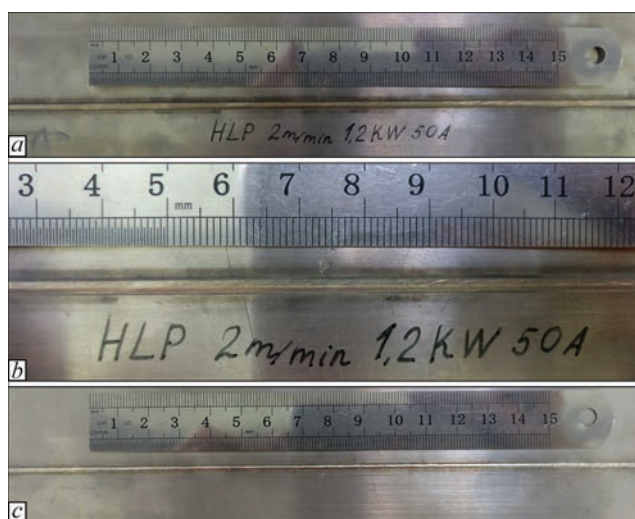
Figure 5. Welded sample of SUS304 ( \delta = 1.5 mm): face (a, b) and reverse (c) sides
