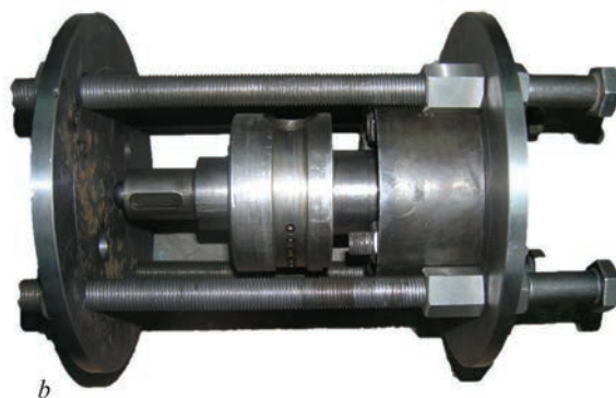
Figure 5. Scheme of beveling the edges of regulator shaft fillet transition ( a ) and fixture for realization of the technology of shaft welding ( b )
