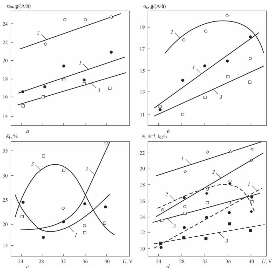
**Figure 2.** Characteristics of melting flux-cored strips depending on voltage (designations are the same as in Figure 1)
