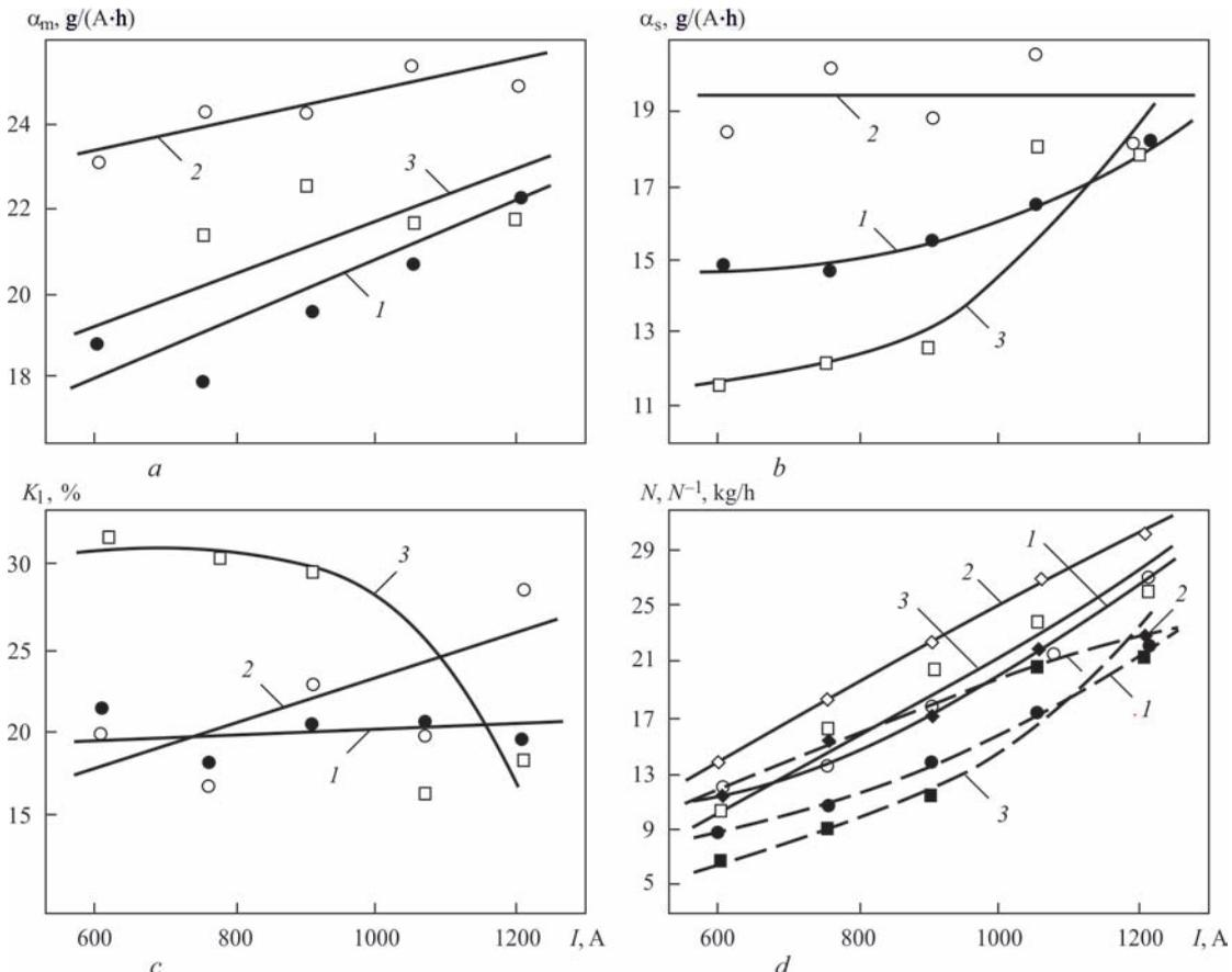
**Figure 1.** Characteristics of melting flux-cored strips depending on current: a — melting factors; b — surfacing factors; c — loss factors; d — efficiency of melting (solid) and surfacing (dashed) of flux-cored strips (1 — PL-AN 101; 2 — PL-AN 111; 3 — PL-AN 179)
