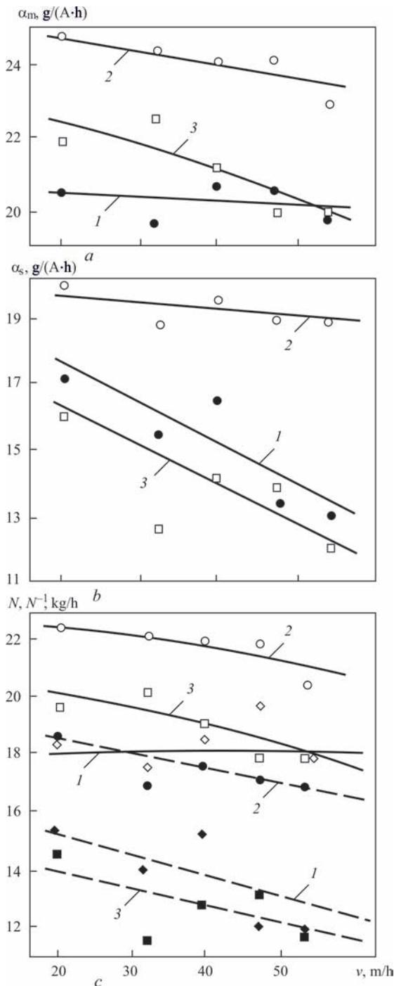
**Figure 3.** Characteristics of melting flux-cored strips depending on change in the rate of surfacing: *a* — melting factors; *b* — surfacing factors; *c* — efficiency of melting (solid) and surfacing (dashed) of flux-cored strips (1 — PL-AN 101; 2 — PL-AN 111; 3 — PL-AN 179)
