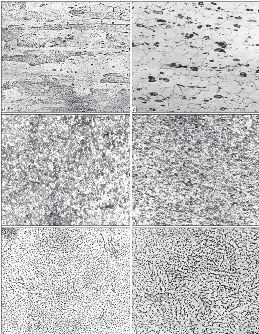
**Figure 3.** Microstructure ( $\times 400$ ) of base metal (*a, b*) and welds (*c–f*) produced at FSW (*c, d*) and automatic TIG welding (*e, f*) of 2 mm alloys 1460 (*a, c, d*) and 1201 (*b, d, f*)
