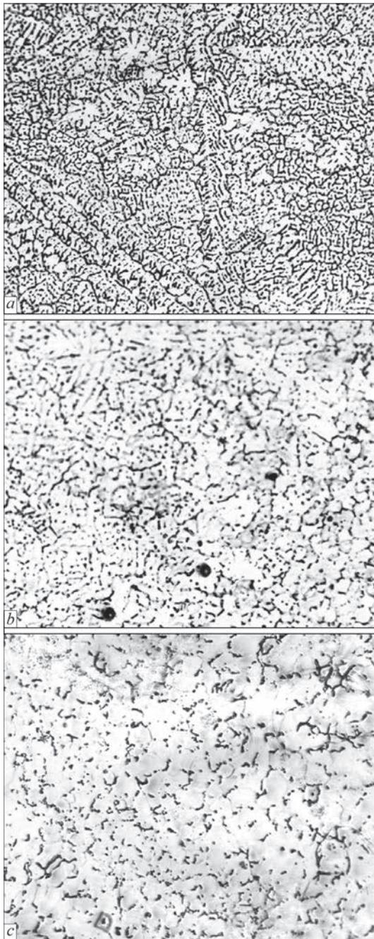
**Figure 1.** Microstructure ( $\times 200$ ) of welds, made by nonconsumable electrode argon-arc welding of 2 mm sheets of alloy 1460 with application of filler wires Sv1201 (*a*) and Sv1201Sc (*b*), as well as arc oscillations, arising at current passing through the section of filler wire Sv1201Sc (*c*)
