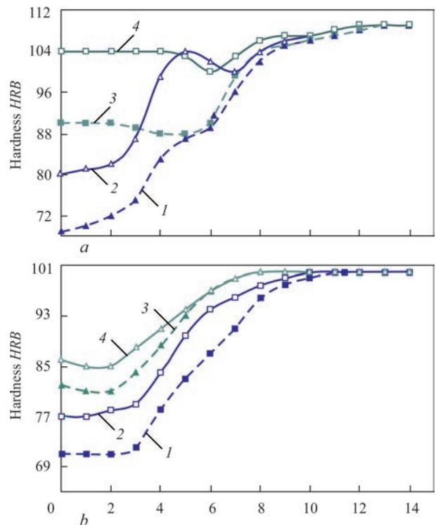
**Figure 4.** Hardness distribution in welded joints of 2 mm alloys 1460 (a) and 1201 (b) produced by automatic TIG welding with arc oscillations with application of filler wire Sv1201Sc and by FSW, directly after welding and after heat treatment of the samples: 1 — Sv1201Sc; 2 — Sv1201Sc (HT); 3 — FSW; 4 — FSW (HT)
