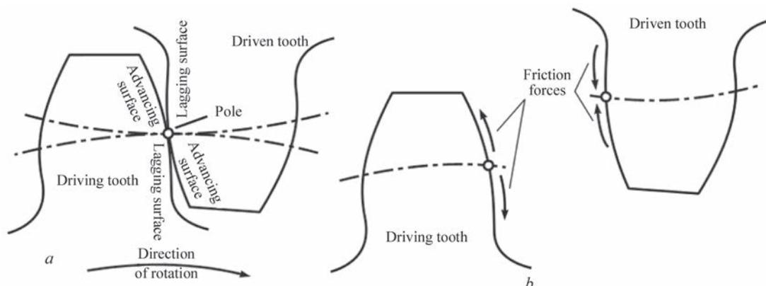
**Figure 4.** Location of lagging and advancing surfaces (*a*) and direction of friction forces (*b*) on driving and driven profiles of the teeth [10]
