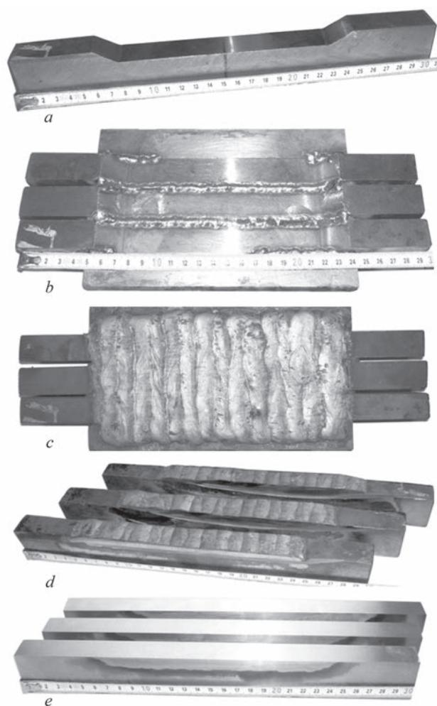
**Figure 3.** Stages of manufacturing deposited specimens: semi-product with a groove for surfacing (*a*); semi-products, assembled into a pack (*b*), after surfacing (*c*), cutting (*d*) and finishing grinding (*e*)
