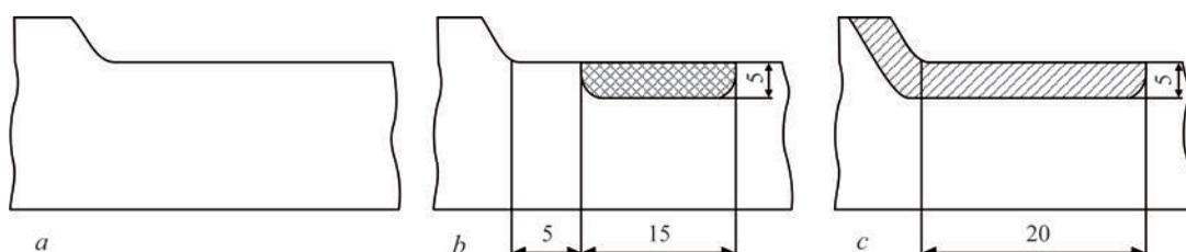
**Figure 7.** Schemes for performing restorative surfacing of specimens for fatigue tests: initial (*a*); with preparation for surfacing according to the scheme 1 (*b*) and with a groove for surfacing according to the scheme 2 (*c*)
