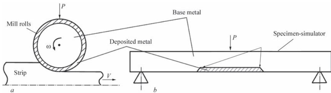
**Figure 1.** Scheme of strip rolling (a) and specimen-simulator loading according to the three-point bending scheme (b). Arrows indicate the transition from base metal to deposited one
