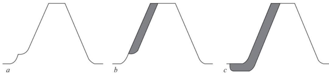
**Figure 5.** Shape of worn tooth (*a*) and possible schemes of its surfacing: *b* — restoration of initial dimensions of a tooth (scheme 1); *c* — restoration-strengthening surfacing with a replacement of damaged material in the stress concentration zone near the tooth root (scheme 2)
