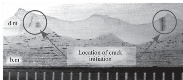
Figure 8. Outer appearance of the side surface of the specimen with the areas where fatigue cracks initiated: b.m. — base metal; d.m — deposited metal
