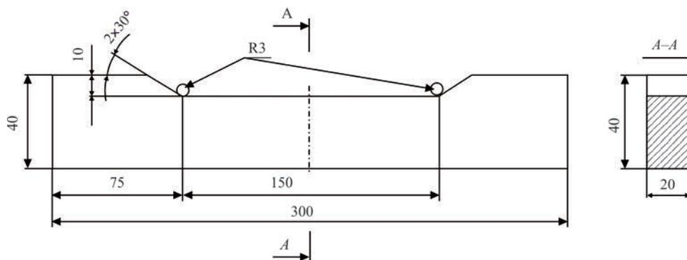
**Figure 2.** Specimen semi-product for investigation of fatigue life with a groove for surfacing with dimensions of 10×20×150 mm
