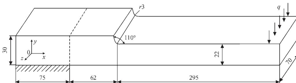
**Figure 6.** Scheme of loading the model specimen for investigation of cyclic fatigue life of a gear tooth (*q* — applied from zero cyclic outer loading)
