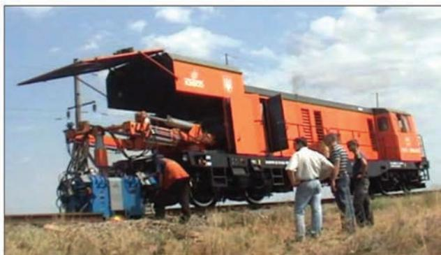
generator, connected with a shaft of power take-off of all-terrain vehicle. Several tens of such mobile welding complexes were successfully used for restoration of railway tracks in hard-to-reach regions of the former USSR railroads.
