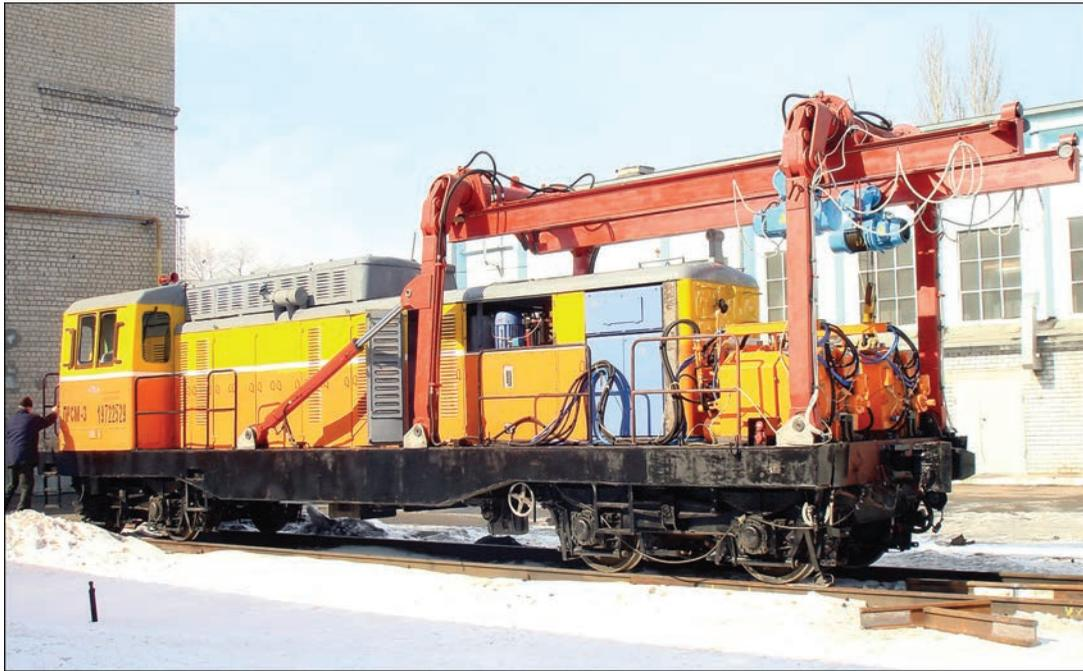
Mobile rail welding complex on railway platform
