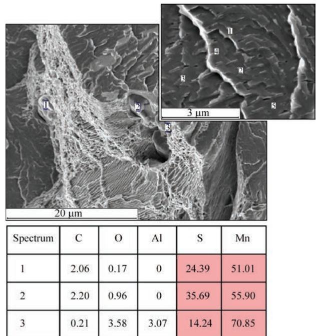
**Figure 7.** Microfractogram of brittle component of fracture surface of ESR rail steel metal
