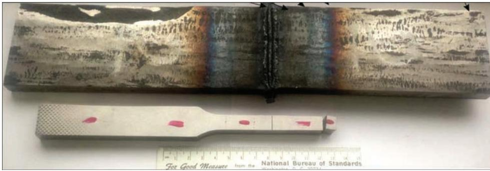
**Figure 2.** Welded butt joints of deformed ESR metal
