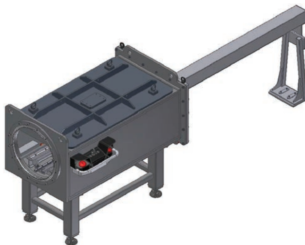
Figure 11. An example of design of auxiliary chamber module for high-productive welding machine
