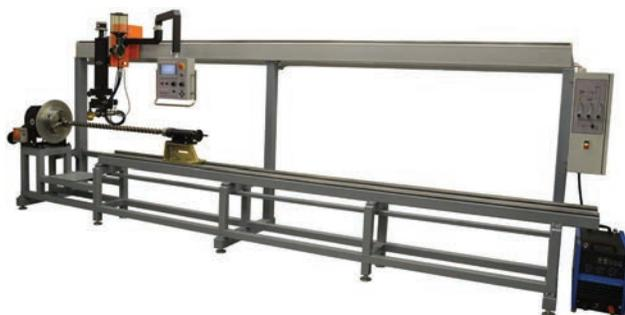
**Figure 11.** Installation RM-70 for PTA surfacing of screws of extruders and automatic molding machines
