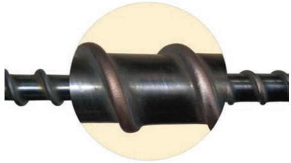
**Figure 13.** Fragment of deposited screw of 63 mm diameter
