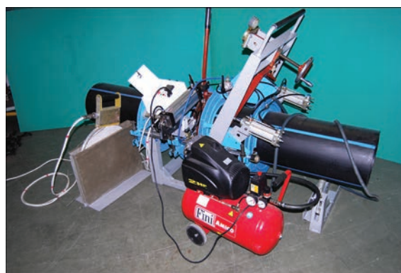
Figure 5. Installation with pneumatic drives for butt welding of polymer pipes of manufacture of the E.O. Paton Electric Welding Institute of the NAS of Ukraine
