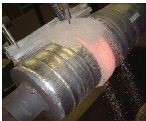
Figure 24. Continuous casting roller cladding with cored wire CHROMECORE 414N-S
