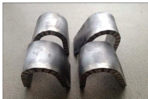
Figure 22. Submerged arc cladding with cored wire EC385. Side bend tests
