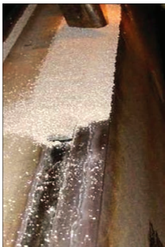
Figure 10. Submerged arc welding with EC316L wire work in the flat position and the weld pool is not visible, it has been developed essentially as an automatic or robotic process.
