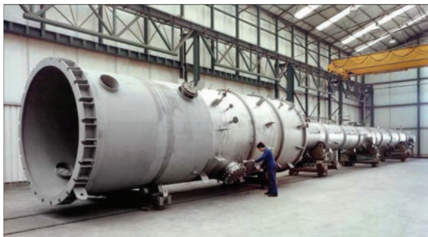
Figure 15. Reboiler in duplex stainless steel FCAW — TETRA S B 22 9 3L-G. SAW — TUBE S 22 9 3L-S + WAF 385
