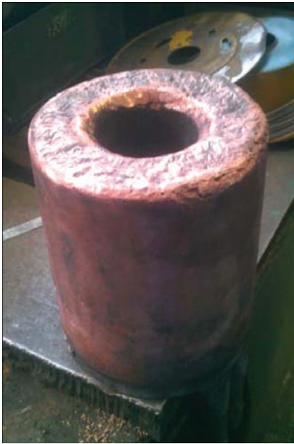
Figure 4. Appearance of restored gas-oxygen chamber diameter of the rings, depending on the type of motor is in the range of 600–1000 mm. The cross-section of workpieces is min 60×20 mm; max is 90×70 mm. The rings are made on rolling units, and then, depending on the diameter, they are welded with one or two butt welds. Figure 2 shows the shape of the butt edge preparation of the workpiece with a section of 90×70 mm.
