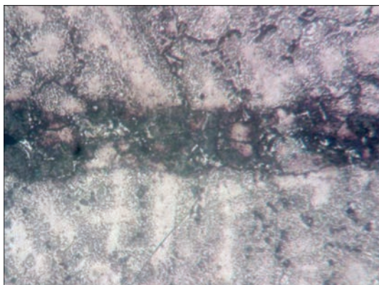
Figure 6. Microstructure ( \times 250 ) of joint of the alloy based on intermetallics \text{Ni}_3\text{Al} in brazing with a constant gap of 0.08 mm by brazing filler metal SBM-3
