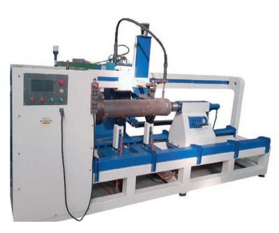
of automatic machines for hardfacing of different spare parts of railway transport (rolls, tails, center bowls, bolsters, side frames of railway bogies).
