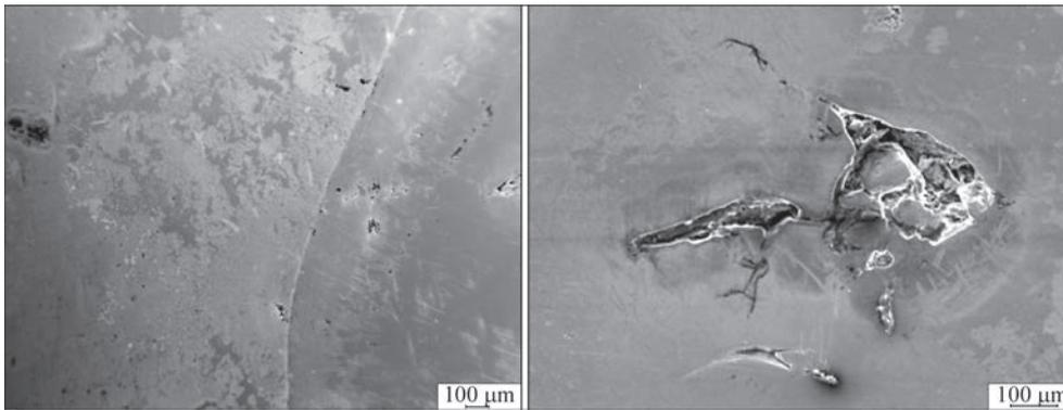
Figure 8. Defects on the surface of sample cross-section
