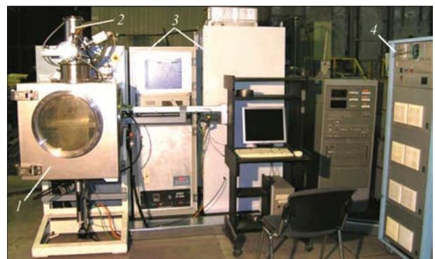
**Figure 2.** Equipment for electron beam 3D printing (for description of 1–4 see the text)
