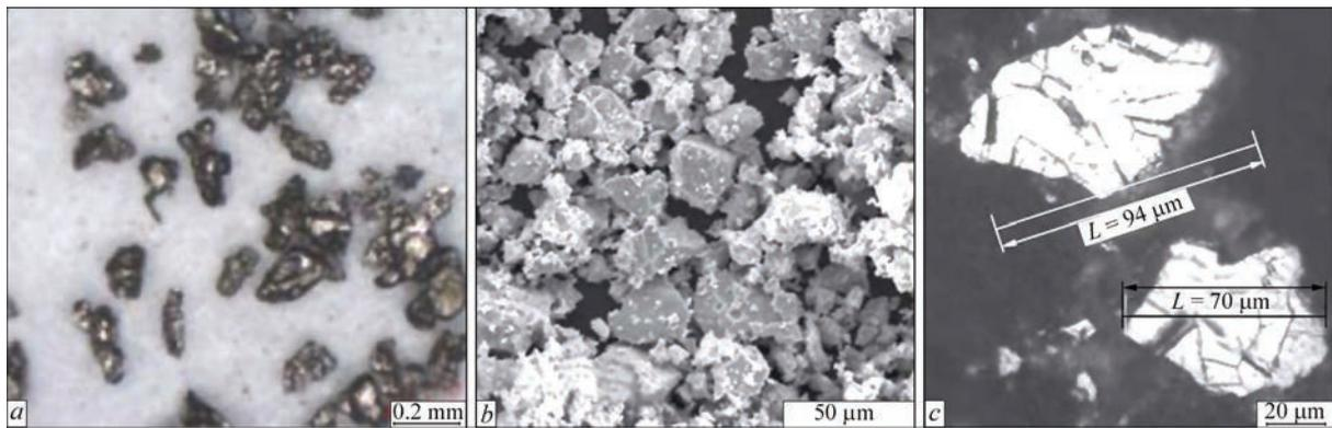
**Figure 1.** Appearance (a) and microstructure (b, c) of HDH VT20 powders with 60 to 140  $\mu\text{m}$  particle size
