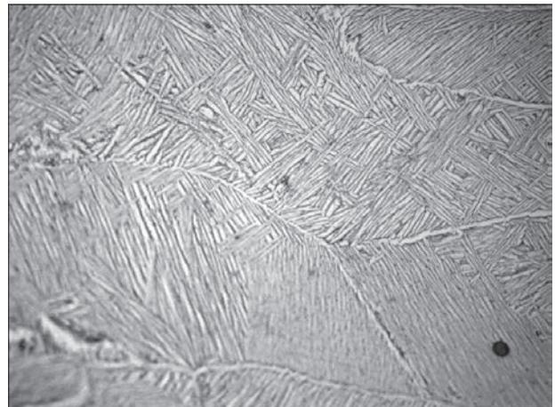
**Figure 11.** Microstructure ( $\times 500$ ) of the deposit metal (VT20 powder)
