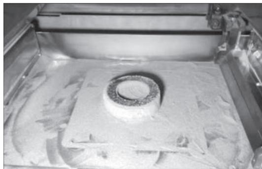
**Figure 5.** Product in vacuum chamber of 3D printer
