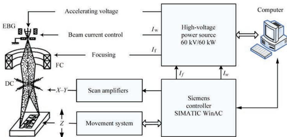
**Figure 4.** Block diagram of control of equipment for additive electron beam fusion: EBG — electron beam gun; FC — EBG focusing coil; DC — EBG deflecting coil (for description of other parameters see the text)
