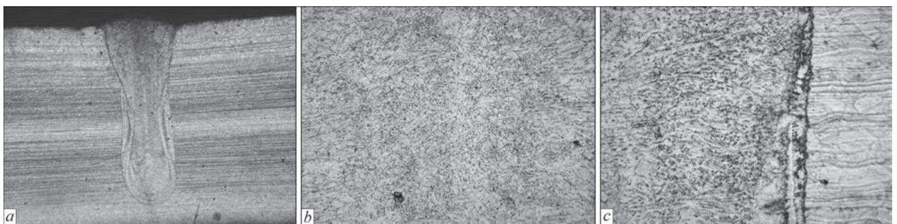
Figure 3. Structure of welded joint metal, made in the flat position: a — cross-section of the weld, \times 30 ; b — center of the weld, \times 400 ; c — fusion line, \times 400
