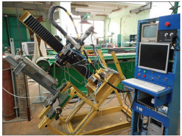
Figure 1. Laboratory bench for laser welding in different spatial positions
