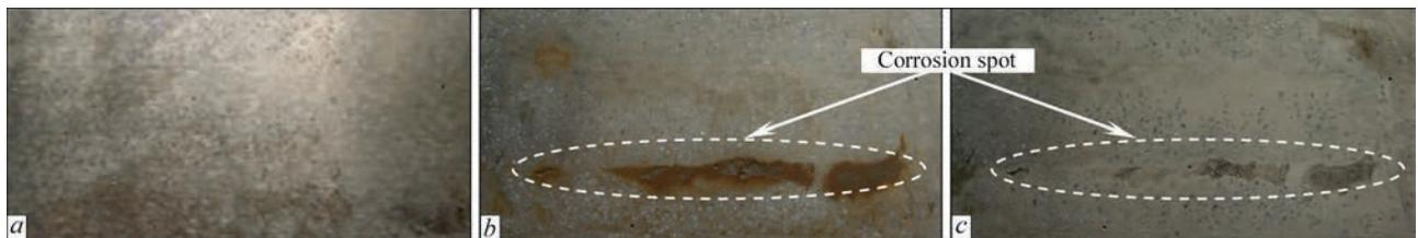
**Figure 3.** Outer appearance of specimen surface of deposited layer on the basis of NiCrBSi: *a* — in the initial state; *b* — with corrosion products; *c* — after removal of corrosion products
