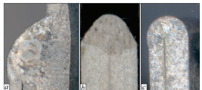
Figure 3. Macrosections of characteristic types of welded joints of cathode unit (CU): a-c — respectively welds No.1, No.5, No.6
