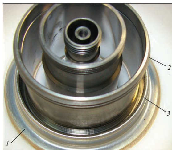
Figure 5. Appearance of CU as-assembled with insulator: 1 — insulator; 2 — CU; 3 — weld
