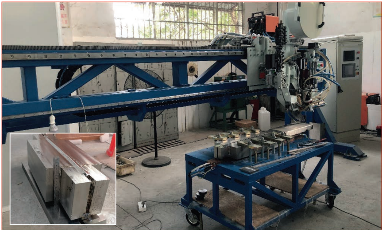
Equipment for narrow gap welding of long-length structures of titanium alloys of 20–120 mm thickness and up to 4 m length and welded product of titanium Ti4–Al–2V alloy of 120 mm thickness under the controlling magnetic field
