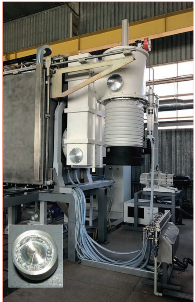
Installation for electron beam welding for application in granular metallurgy
