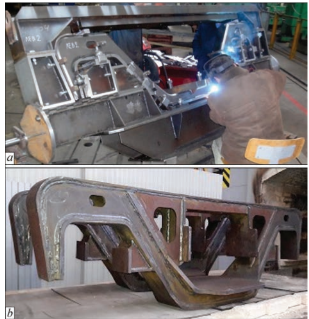
Figure 4. Equipment for assembly and welding of side frame structure ( a ) and two manufactured test specimens ( b )
