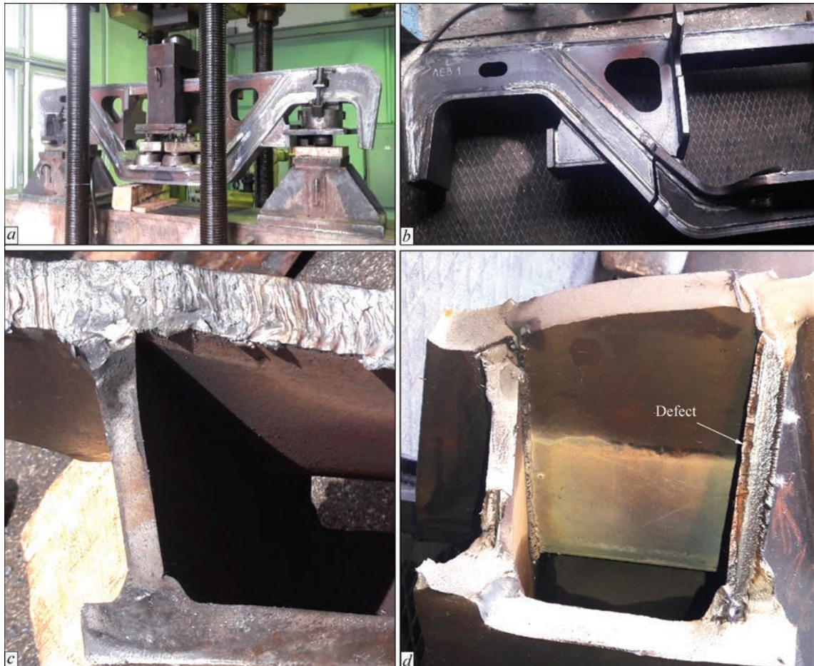
Figure 5. Test specimen No.1 of all-welded side frame during accelerated fatigue tests ( a ) and fracture in the area of transverse welded joint of side wall ( b ), fracture in the zone of a first crack ( c ) and in the fracture zone ( d )
