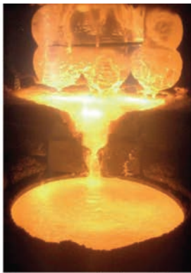
Remelting sponge titanium briquettes into 400 mm diameter ingot of Grade 2
