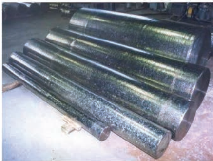
Titanium ingots of 100–600 mm diameter
