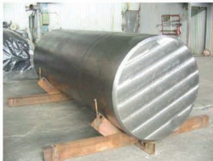
Titanium ingot of 1100 mm diameter
