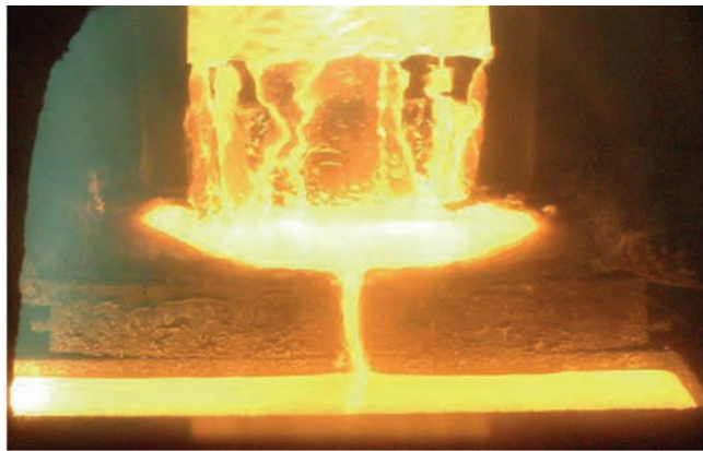
Producing 165×950×2500 mm slab-ingot of PT-3V titanium alloy
