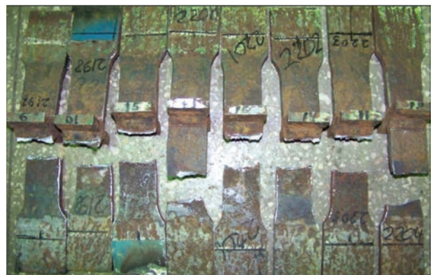
Fig re 5 Specimens of T-welded joints of 15KhSND steel with surface fatigue cracks, which were strengthened by HFMP after soaking for 1200 h in KST-1 chamber, shown after fatigue testing
