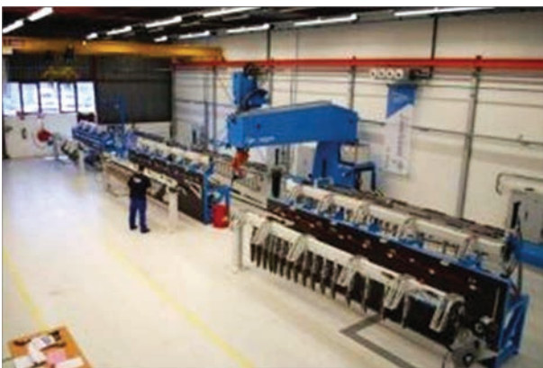
Fig re 3 Production of elevating rudders and yaw rudders by the method of induction welding from TPC carbon fiber/PPS for Dassault Falcon 5X jet aircraft
