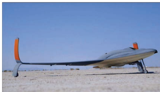
Fig re 9 UAV in which 80 % of parts are printed of polymer materials
