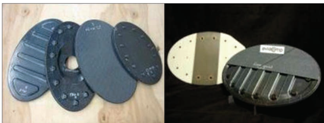
Fig re 4 Fuel tank access hatches for narrow Airbus A220 aircrafts, made of TPC by the Company Aviacomp using induction welding technology developed by the Company KVE Composites
