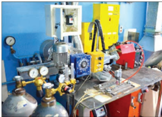
Figure 1. Stand for arc (plasma) brazing
