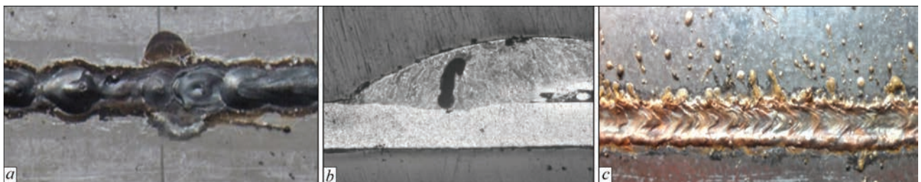
Figure 3. Appearance ( a ), and macrostructure ( b ) of the weld produced by MIG-welding and MIG-brazing ( c ) of galvanized steel
