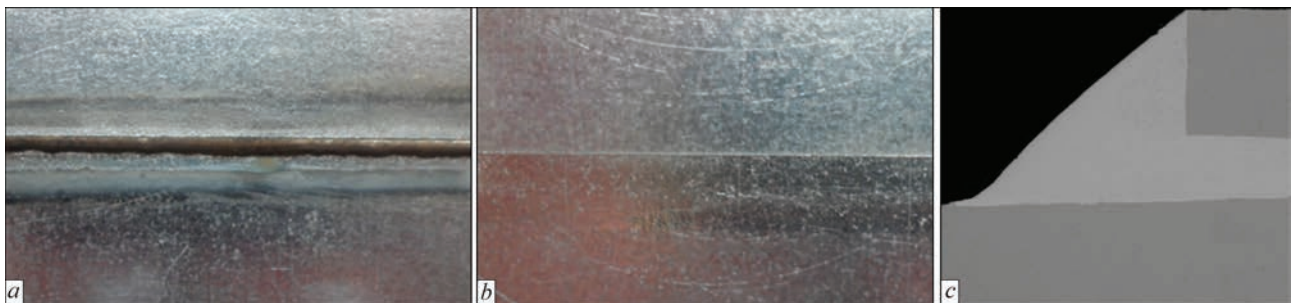
Figure 6. Face (a), back side (b) and macrostructure (c) of brazed overlap joint of galvanized steel
