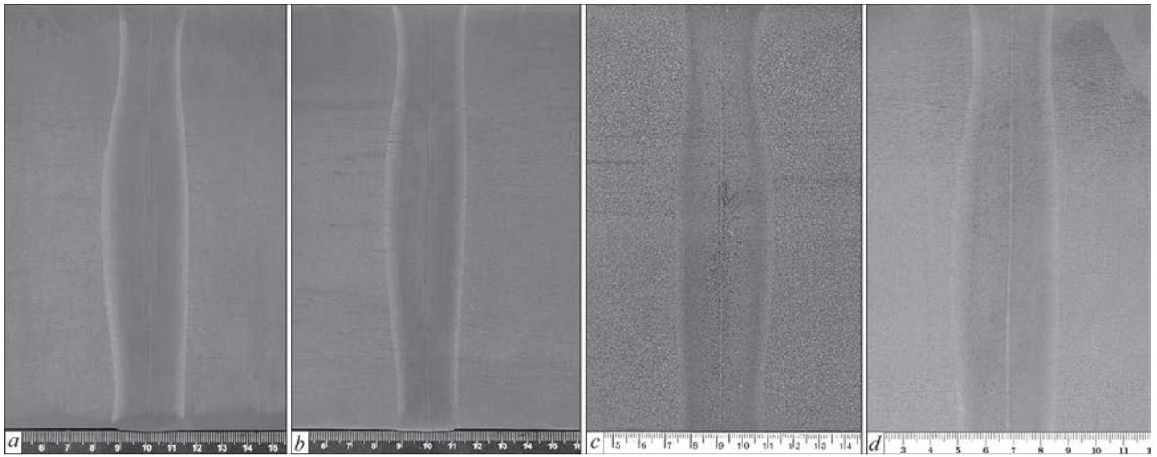
**Fig re 4** Macrosections of rails of different steel grades in pulsed flash-butt welding in the optimum modes *a* — R350HT (HAZ — 28 mm); *b* — K76F (HAZ — 27 mm); *c* — R260 (HAZ — 31 mm); *d* — M76F (HAZ — 37 mm)
