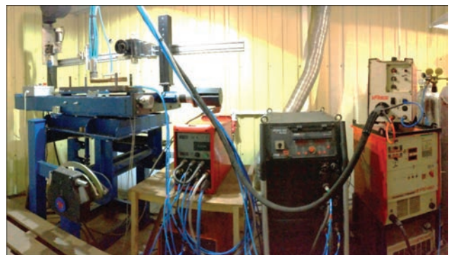
Fig re 3 Appearance of laboratory complex of Plasma-MIG welding
