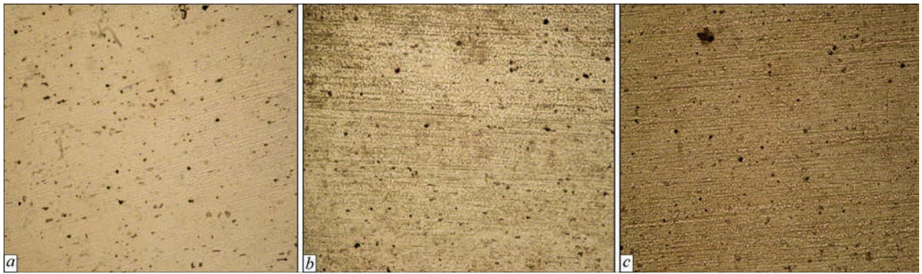
Fig re 1 Microstructure ( \times 320 ) of base metal of V1341 alloy in the state after quenching and natural ageing (a), after artificial ageing (b) and after complete heat treatment (quenching and artificial ageing) (c)
