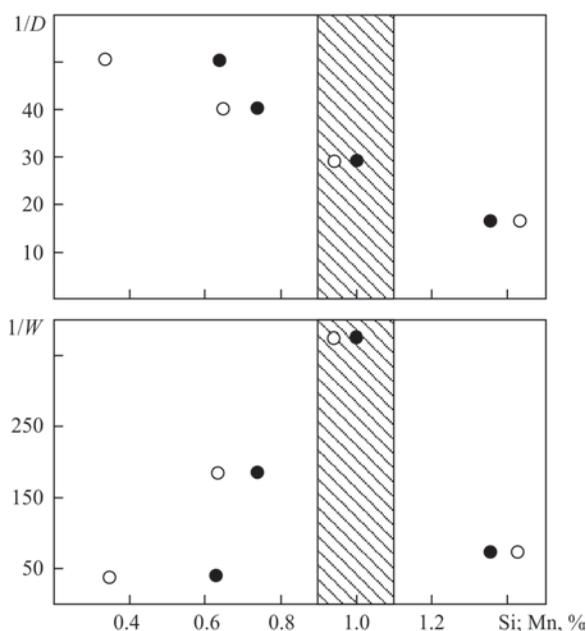
**Fig re 4** Dependence of resistance to damage and wear on silicon and manganese content, as well as their recommended content (shaded area)
