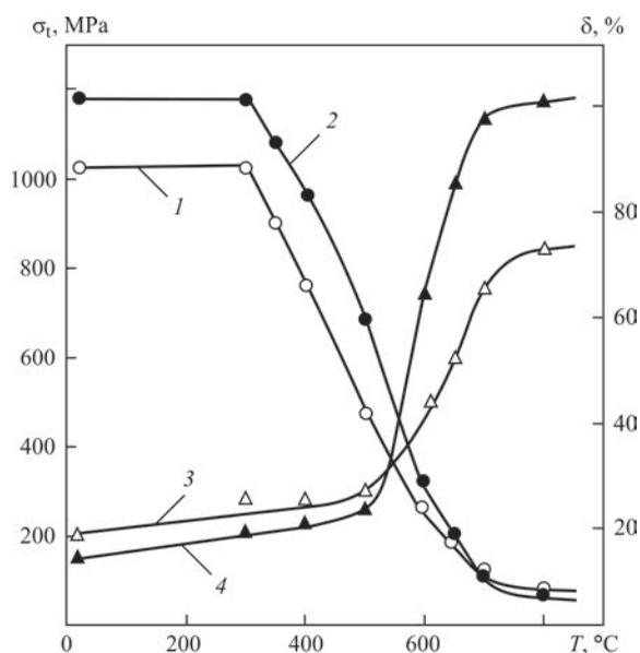
**Fig re 2** Temperature dependence of strength (1, 2) and ductility characteristics (3, 4) of steels of grades 2 (1, 3) and T (2, 4)
