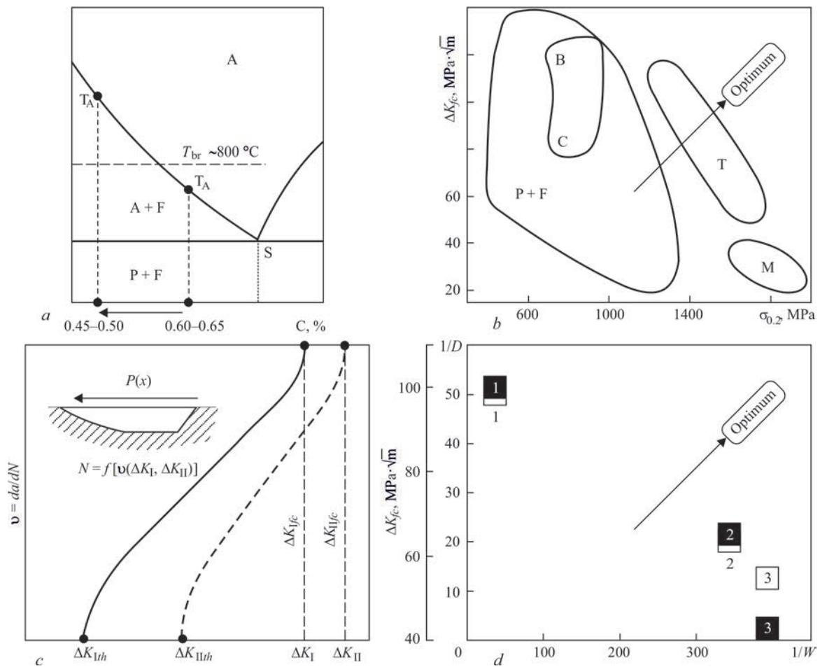
**Fig re 1** New concept of creating high-strength wheel steels:  $T_A$  — austenitization temperature;  $T_{br}$  — temperature in the area of wheel-rail contact during braking; A — austenite, F — ferrite, P — pearlite, B — bainite, M — martensite, T — troostite, S — sorbite; 1 — steel of grade 2, 2 — of grade T, 3 — of grade  $T_m$ . Light symbols – diagram  $(1/D - 1/W)$ ; dark –  $(\Delta K_{I/c} - 1/W)$ ; description a–d see in the text
