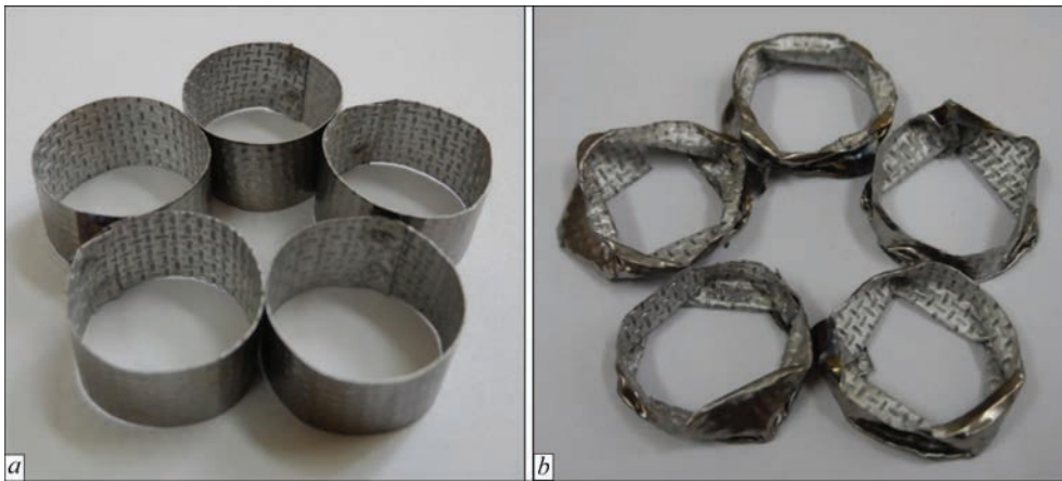
Figure 5. General view of cylindrical samples before (a) and after (b) compressive testing
