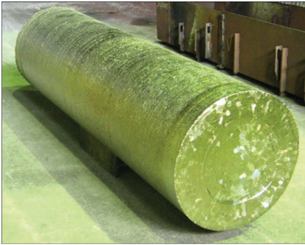
Figure 3. Ingot of Grade 3 titanium alloy of 600 mm diameter after EBCHM
