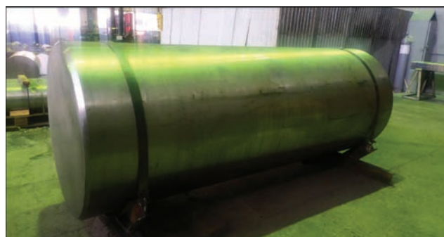
Figure 4. Appearance of an ingot of Grade 3 titanium alloy of 1100 mm diameter after machining
