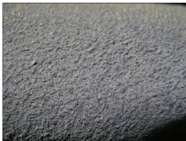
Figure 12. Macrostructure of sprayed tubes after six years of operation
