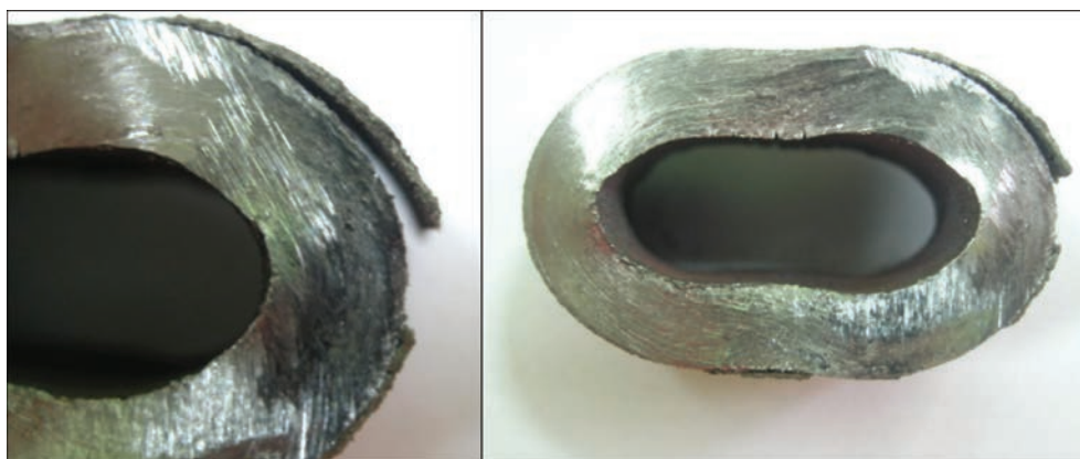
Figure 10. Specimens after tests on flattening
