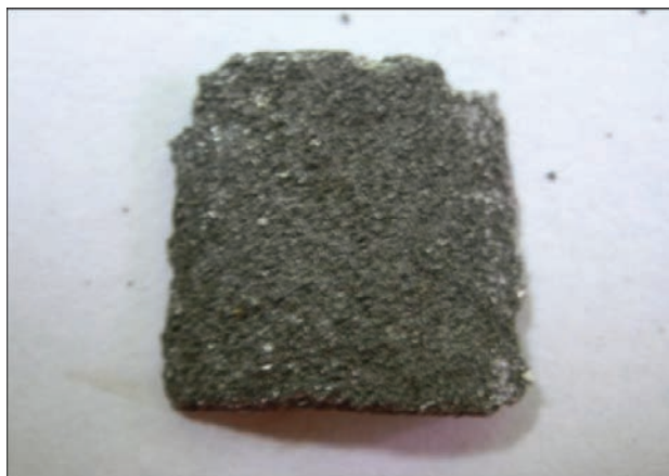
Figure 11. Delaminated layer after test on flattening
