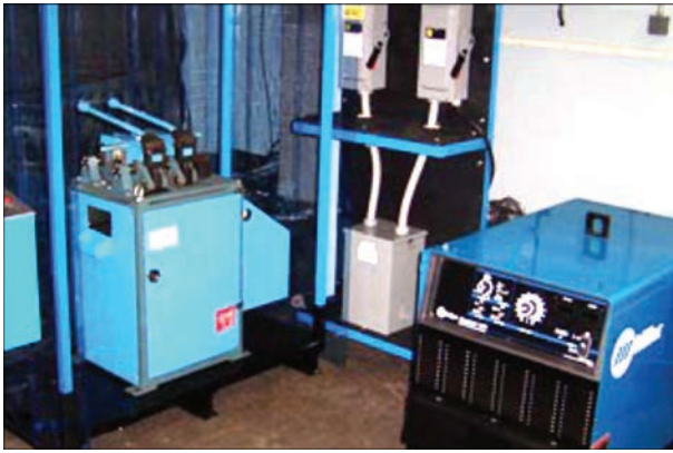
Figure 2. MD-101 machine for MIAB welding of pipes
