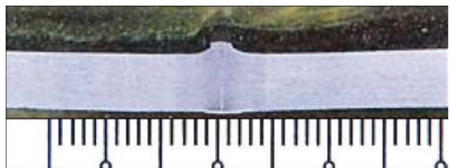
Figure 9. Welded joint macrosection
