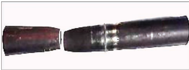
Figure 5. Rupture testing of a welded pipe sample
