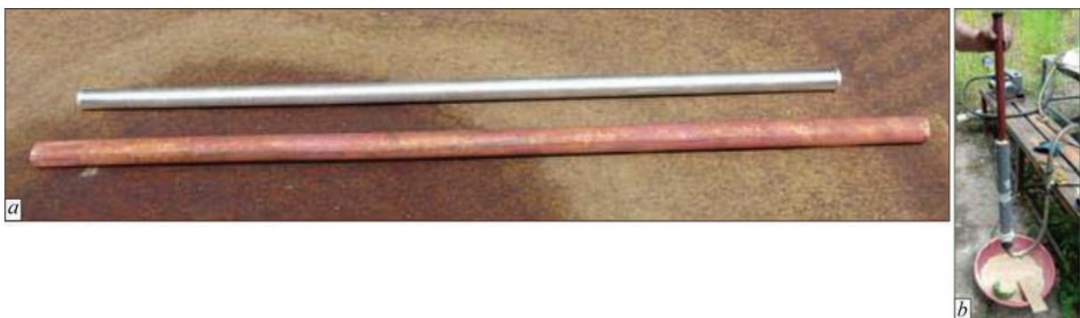
Figure 2. Workpieces for explosion welding (a), loading of explosives into a folded container (b)
