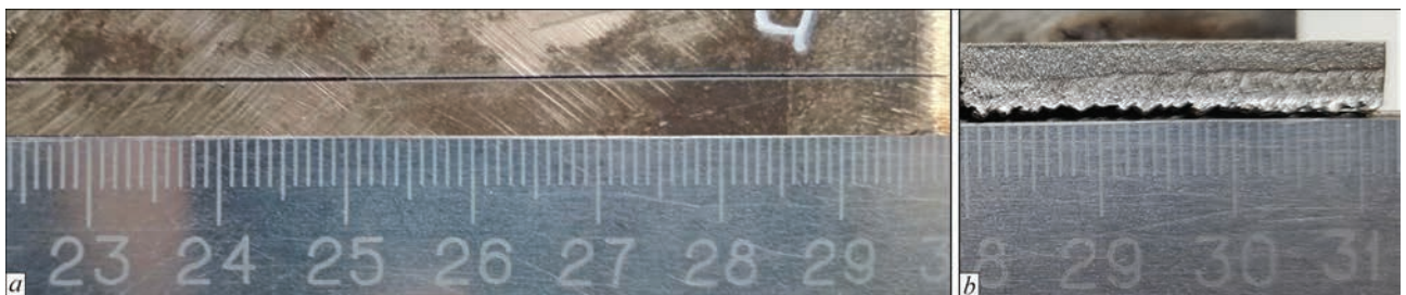
Figure 3. Width (a) and edge (b) of a laser cut of shaped pipe from steel of Q235 type (5 mm wall thickness)
