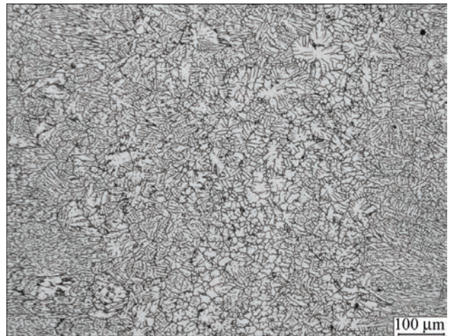
Figure 5. The microstructure of the equiaxed dendrite zone in the weld metal centre ( I_b = 60 mA, v = 50 mm/s)
