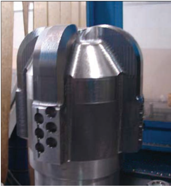
Figure 4. Frame of an integrally-milled bit
