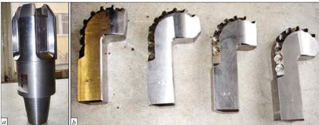
Figure 5. Combined bit: a — frame; b — blades
