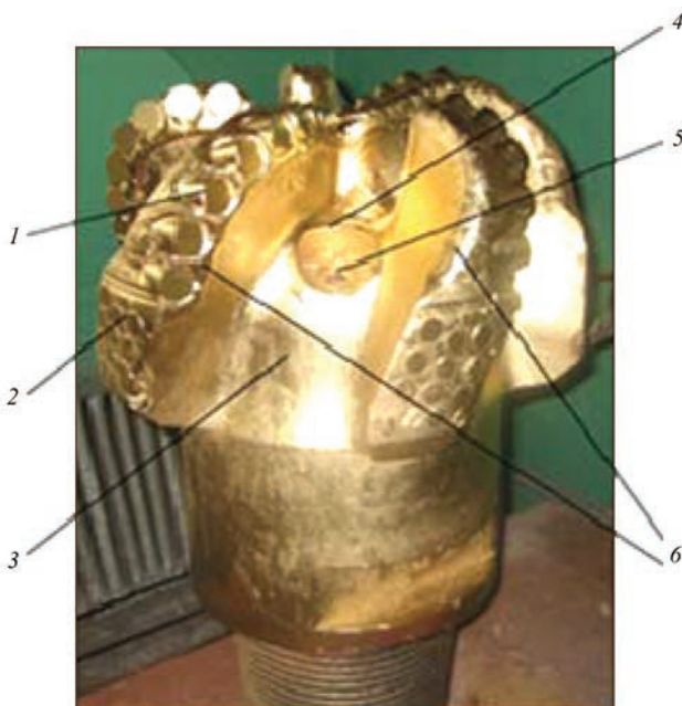
Figure 1. Scheme of arrangement of working bodies of a bit: 1 — cutter; 2 — hard-alloy insert of calibration surface; 3 — interblade space for sludge removal; 4 — protective coating of watercourse; 5 — hard-alloy nozzle of watercourse; 6 — protective coating of working bodies of blades
