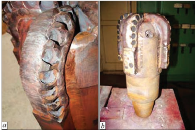
Figure 6. Deposition of coating on working bodies of a bit: a — blade; b — bit after brazing of diamond-hard-alloy cutters and inserts
