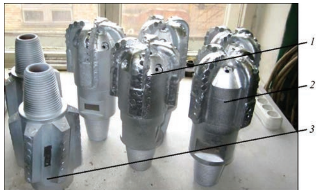
Figure 8. Drill bits with a protective coating: 1 — combined bit; 2 — integrally-milled bit; 3 — calibrator
