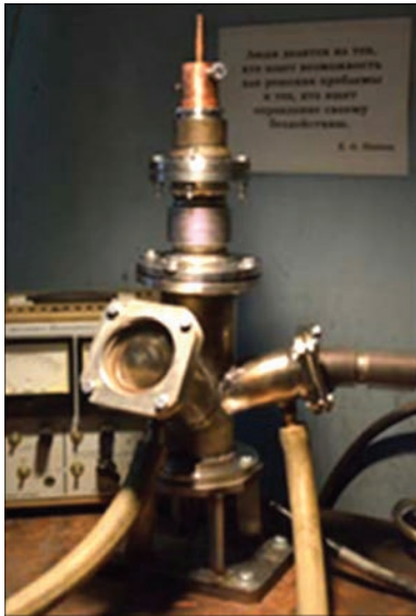
Figure 1. Laboratory installation for melting brazing filler metals in argon
