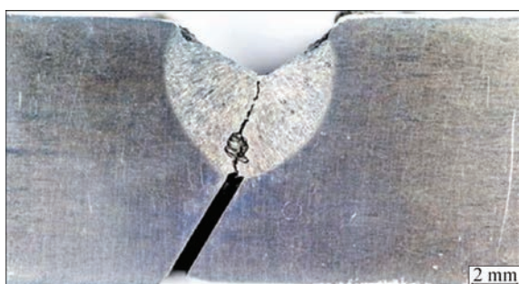
Figure 2. Cross-section of an underwater weld [11]
