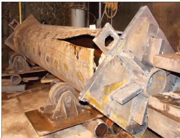
Figure 4. General view of the site of fracture in a pipe reference specimen after hydraulic loading by pressure 13.25 MPa
