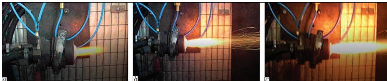
Figure 6. Appearance of plasma jet: a — at absence of powder feed without magnetic field; b — powder feed without magnetic field; c — powder feed with magnetic field
