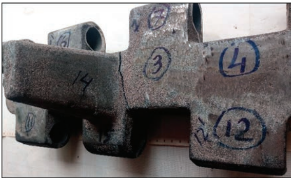
Figure 7. General view of integrity loss (crack formation) of metal of tracks 1–4 (2021) after 4-point bend tests
