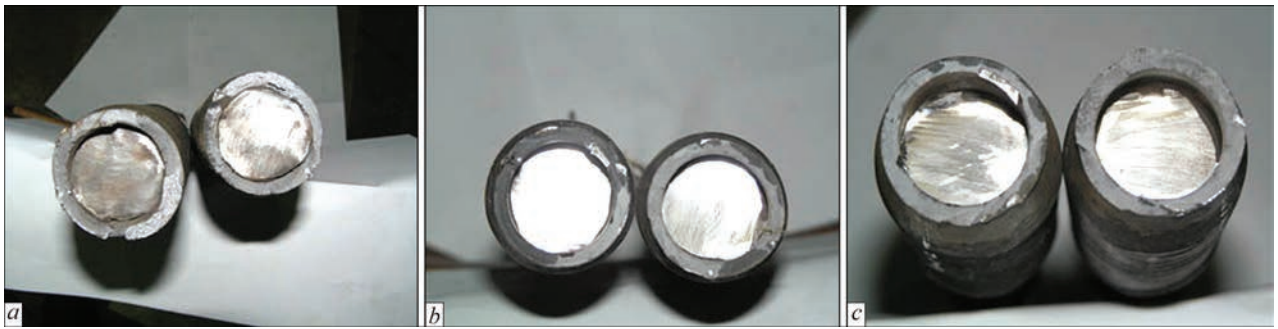
Figure 4. Nature of fracture of samples during tensile tests: a — sample with a zero gap; b — sample with a gap of 20 mm; c — sample with a gap of 40 mm
